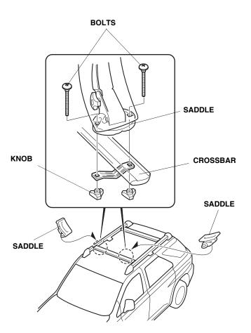
Position the two hydro-glide assemblies on the rear crossbar. Loosely install the hydro-glide assemblies using one bracket, two bolts, and two knobs for each assembly. The distance between the two assemblies should be the same width as the kayak.
