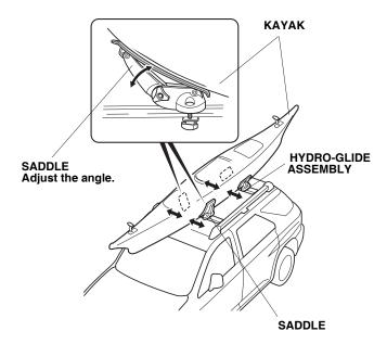
Slide the kayak forward or backward until it's level with the roof. If necessary, loosen the knob on each saddle and adjust the saddle angle to fit snugly against the kayak. Tighten each knob securely. 6. Route each strap with buckle through the buckle cover with the ribbed side facing up.
