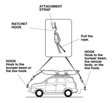
13. To loosen the rope, push up on the ratchet strap lever, then pull on the other end of the rope.
