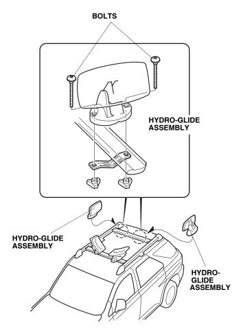
Rest the front of the kayak on the hydro-glide assemblies. Standing behind or alongside the kayak, lift up the rear of the kayak and push it forward onto the hydro-glide assemblies and saddles. Make sure the kayak reaches the front saddles before you lower it
